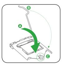
Insert the load lever under the retention tab.
